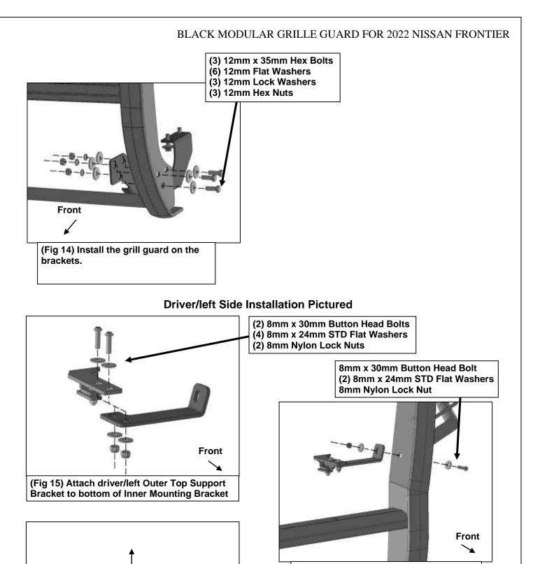
(Fig 16) Attach driver/left Top Support Bracket to inside of Grille Guard upright
