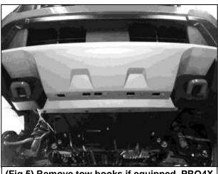
(Fig 5) Remove tow hooks if equipped. PRO4X model not equipped with splash guard pictured from below
