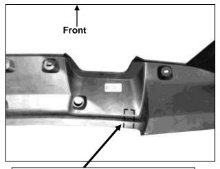
(Fig 18) Cut slots to clear the Brackets (passenger/right side pictured, dashed line for example only)
