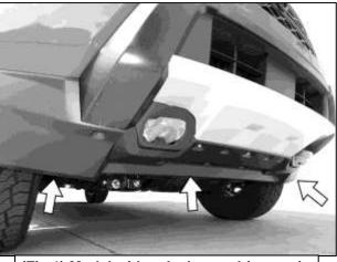
(Fig 1) Model with splash guard (arrows)
