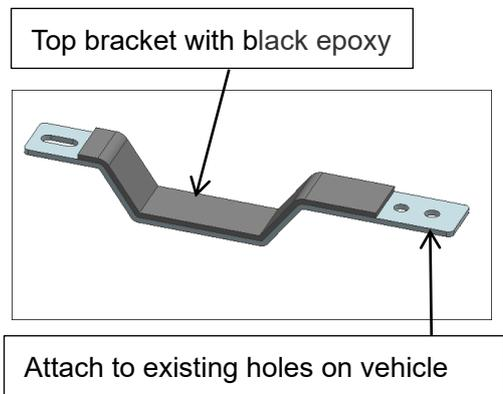
**INSTALLING THE FRAME BRACKETS**
