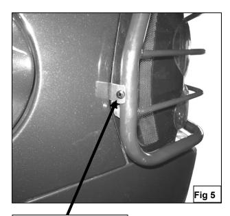
4mm x 15mm Phillips Screw 4mm Lock Washer 4mm Flat Washer
