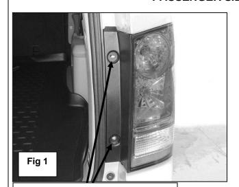
To remove taillight assembly, unscrew the two hex bolts, firmly grasp taillight assembly and pull evenly, straight back from vehicle. Do not pry assembly from vehicle or damage may result.
