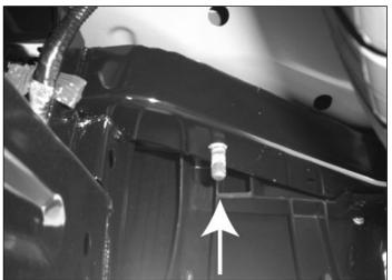
**3.** Insert (1) 1/2" bolt with rod extension through outside opening in square cross member and position so threaded end drops through hole in cross member. **Passenger side shown**
