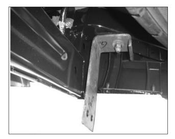
**4.** Fasten bumper bracket to cross member using (1) 1/2" locknut and (1) 1/2" flat washer. Tighten until slightly snug. Repeat for opposite side. **Passenger side shown**
