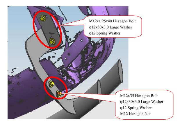
Step 3: Install the rear guard on the brackets and then adjust them to the proper positions.
