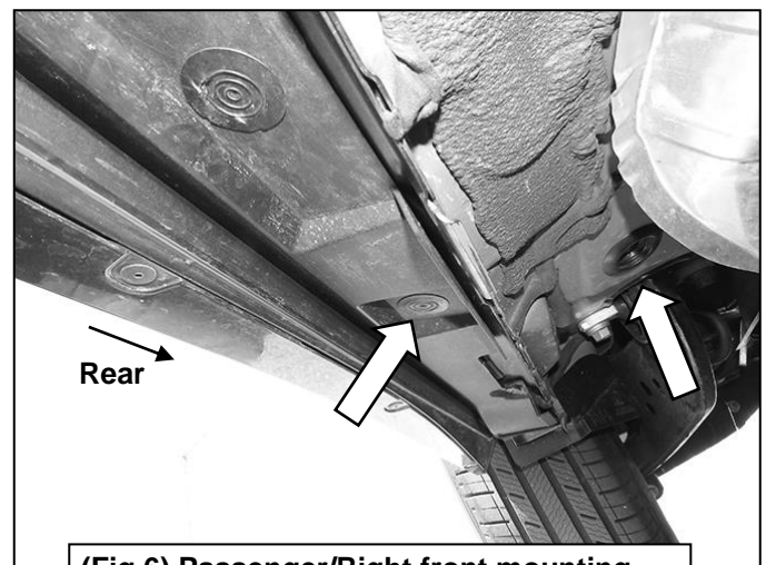
(Fig 6) Passenger/Right front mounting location, Remove plastic plugs from holes
