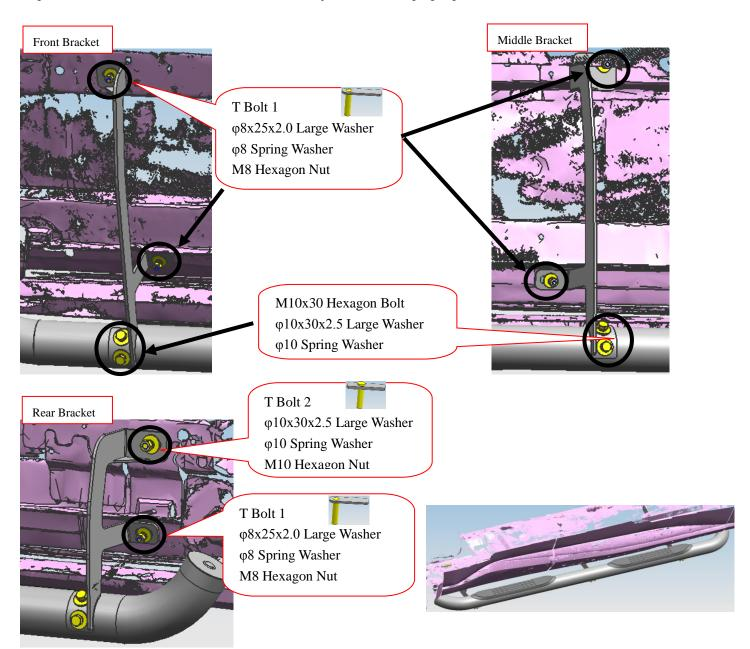
Step 4: Check if all hard ware are installed and then fasten all to complete the installation.
