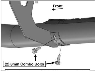
(Fig 22) Passenger/Right Sidebar installation
