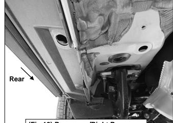
(Fig 18) Passenger/Right Rear mounting location (Plastic covers removed for instruction purposes)
