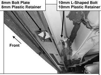
(Fig 16) Insert 8mm Bolt Plate and 10mm L-Shaped Bolt into the Passenger/Right Center mounting holes
