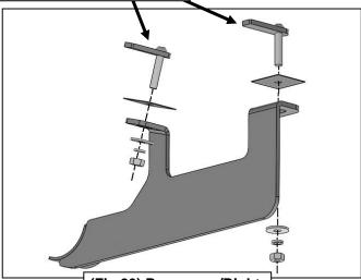
(Fig 20) Passenger/Right Rear Bracket installation
