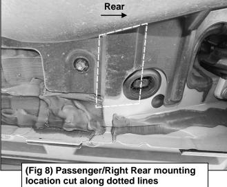
IMPORTANT: Cut the plastic covers enough to allow the mounting brackets to mount against the body
