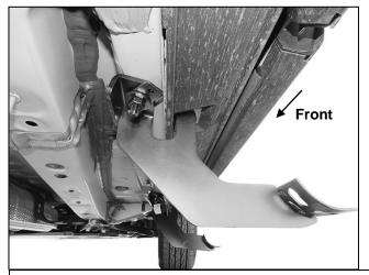
(Fig 17) Passenger/Right Center Bracket installed
