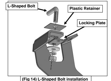
10mm L-Shaped Bolt 10mm Plastic Retainer Locking Plates 10mm Flat Washer 10mm Lock Washer 10mm Hex Nut
