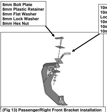
10mm L-Shaped Bolt 10mm Plastic Retainer Locking Plate 10mm Flat Washer 10mm Lock Washer 10mm Hex Nut
