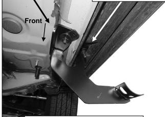
(Fig 15) Passenger/Right Front Bracket installed (Plastic covers removed for instruction purposes)
