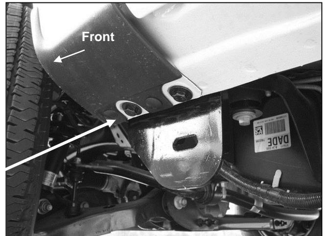
(Fig 2) Driver side front Mounting Bracket pictured
