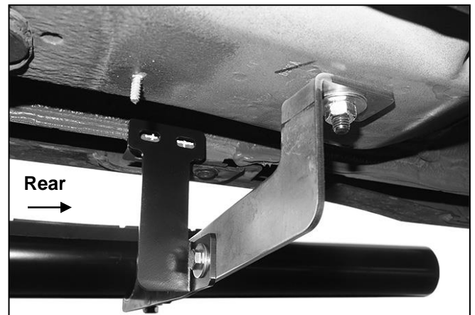
(Fig 11) Mark back of pinch weld to drill for Support Bracket (Passenger rear Support)
