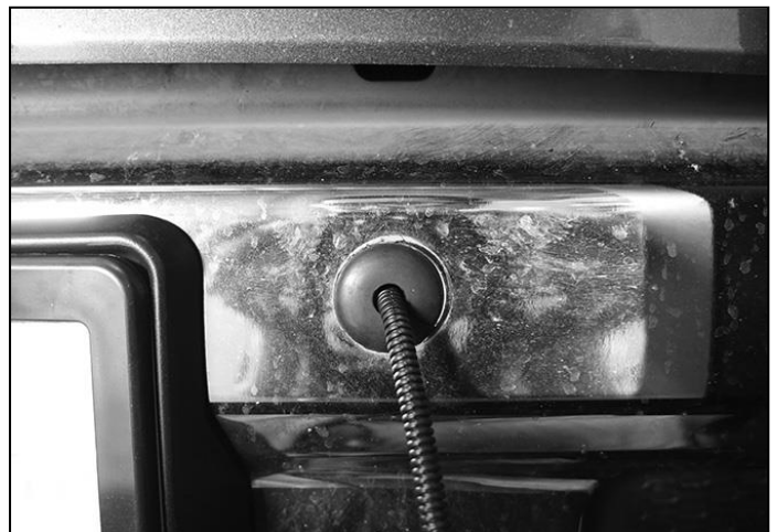
(Fig 20) Models with sensors, slide Grommet over small end of Harness Extension. Push Grommet into hole in bumper and attach to wiring harness
