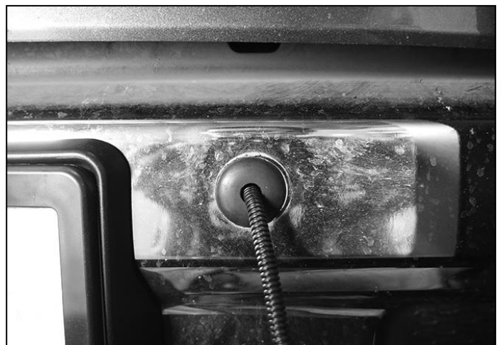
(Fig 20) Models with sensors, slide Grommet over small end of Harness Extension. Push Grommet into hole in bumper and attach to wiring harness
