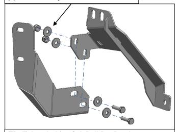
(Fig 5) Attach driver/left Bull Bar Bracket to outside of Mounting Bracket
