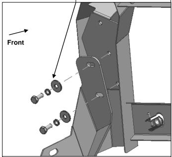
(Fig 10) Attach Bull Bar Bracket to back of Bull Bar
