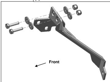
(Fig 2) 2021 models only :Attach driver/left Frame Bracket to bottom of frame. Attach skid plate bracket to rear mounting bolt if equipped with steel skid plate
