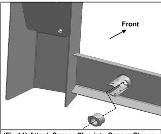
(Fig 11) Attach Sensor Plug into Sensor Sleeve
