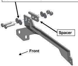
(Fig 3) 2022-on models only: Insert Spacer between top of Bracket and mounting tab. Reuse the factory hex nut to attach the bottom of the Bracket to the crossmember. Driver/left Bracket illustrated.
