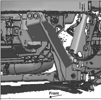
(Fig 4) Driver/left Frame Bracket installed with optional Skid Plate Bracket (arrow)
