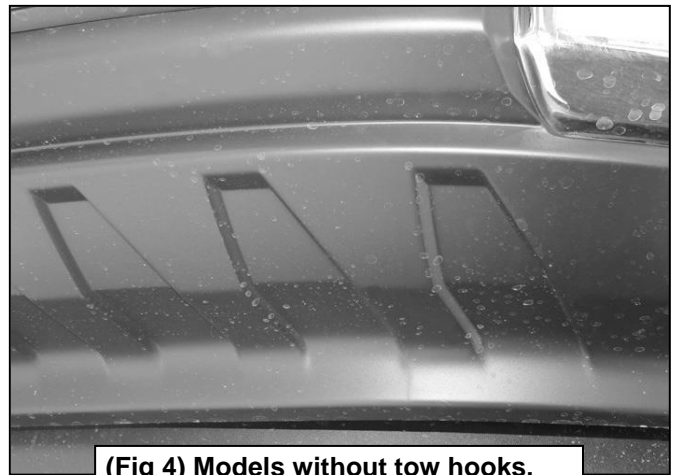
(Fig 4) Models without tow hooks, temporarily remove the plastic splash guard and spoiler if equipped
