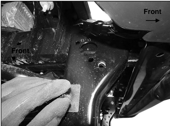
(Fig 3) Use Retainer to hold 10mm Bolt/Nut Plate. Rotate Bolt/Nut Plate to line up Nut with factory hole
