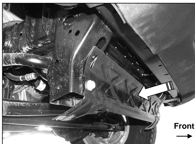
(Fig 1) Remove splash guard and bracket (arrow)
