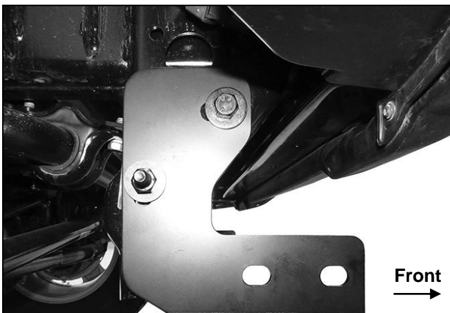
(Fig 5) Passenger/right Frame Bracket installed
