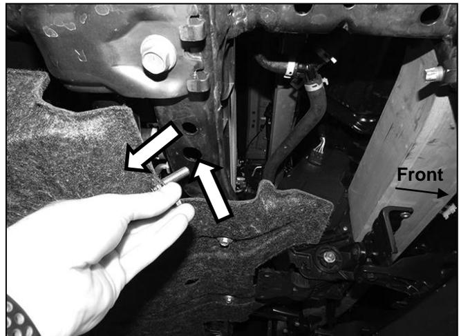
(Fig 4) Insert (1) 10-1.5mm x 35mm Bolt Plate with Fish Wire into the large hole on the crossmember and out the smaller hole towards the side of the vehicle
