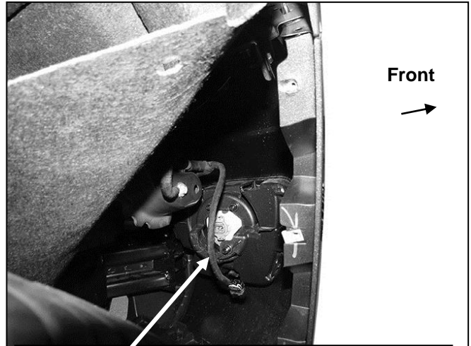
(Fig 7) Pull back fender liner to access bumper hardware and unplug fog light if equipped
