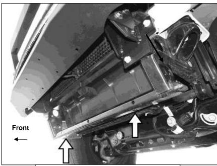
(Fig 1) Attach Skid Plate to back of Bumper and bottom of cross member (arrows)
