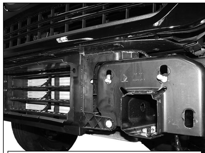
(Fig 3) Remove bumper (driver/left side pictured)
