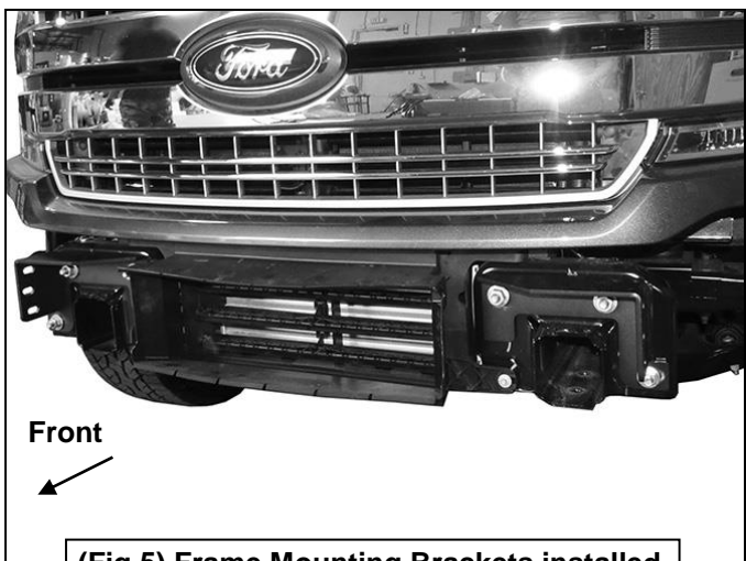
(Fig 5) Frame Mounting Brackets installed
