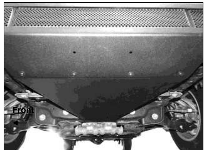
(Fig 4) Skid Plate attached to Bumper
