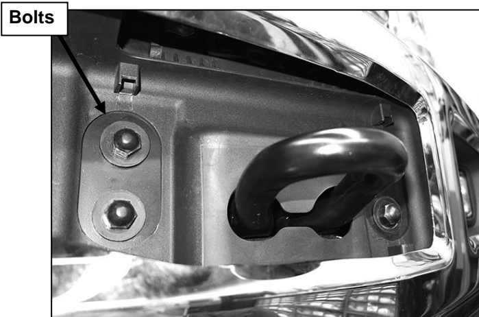
(Fig 4) Remove bumper bolts (driver side pictured)
