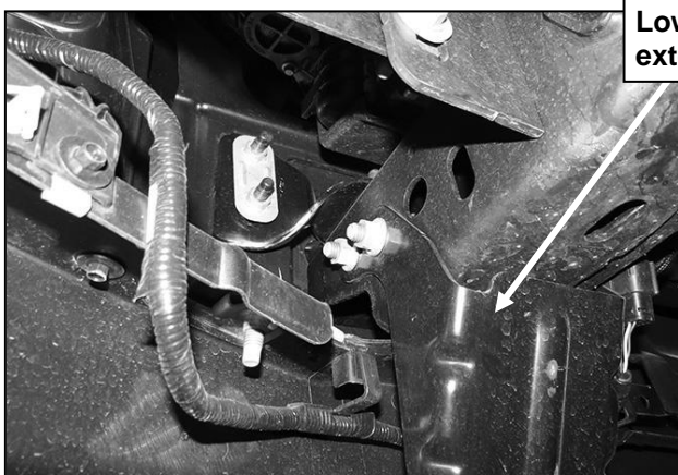
(Fig 1) Driver side lower frame extension and fog light wire harness pictured from behind bumper
