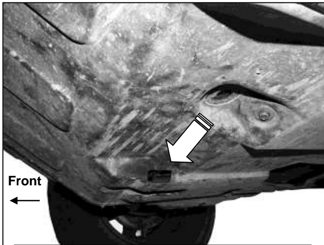
(Fig 4) Reinstall splash guard. Note insert flat passenger/right side of Bracket through slot and between skid plate and crossmember
