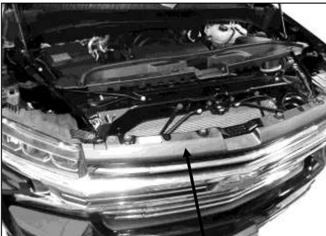
(Fig 1) Remove cover and screws attaching grille
