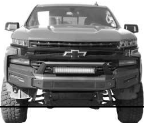
(Fig 18) Reuse factory hex bolts to attach Bumper to end of frame
