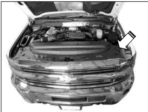
(Fig 1) Remove plastic cover and grille
