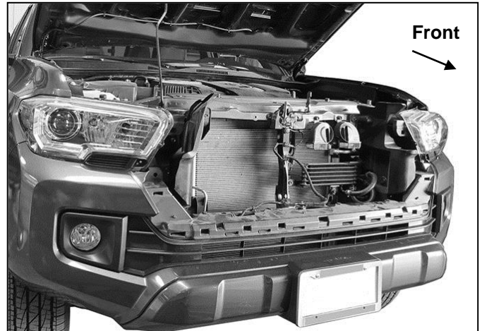
(Fig 2) Remove grille, air dam from below bumper and license plate. Remove plastic bumper cover
