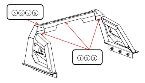
**Step2:** Place the roll bar on the truck in an appropriate location.
