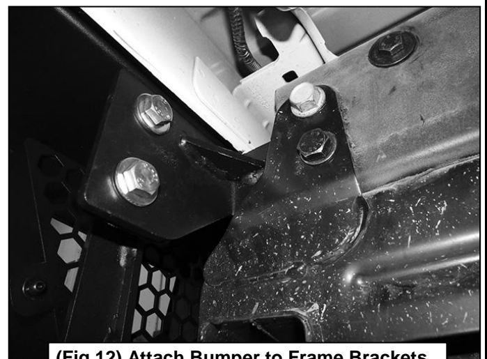
(Fig 12) Attach Bumper to Frame Brackets
