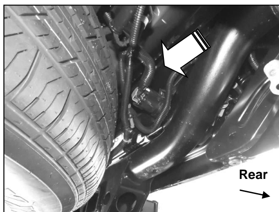
(Fig 4) Unplug the trailer plug (arrow)
