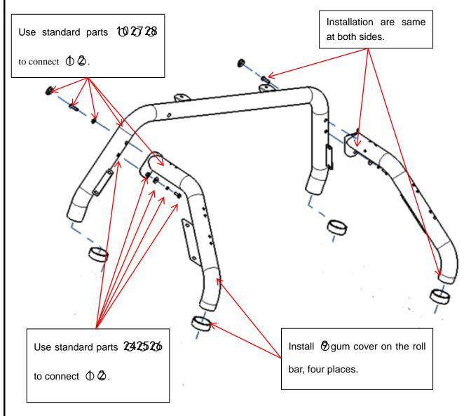
**Step2:** Install the roll bar and luggage frame as following picture.
