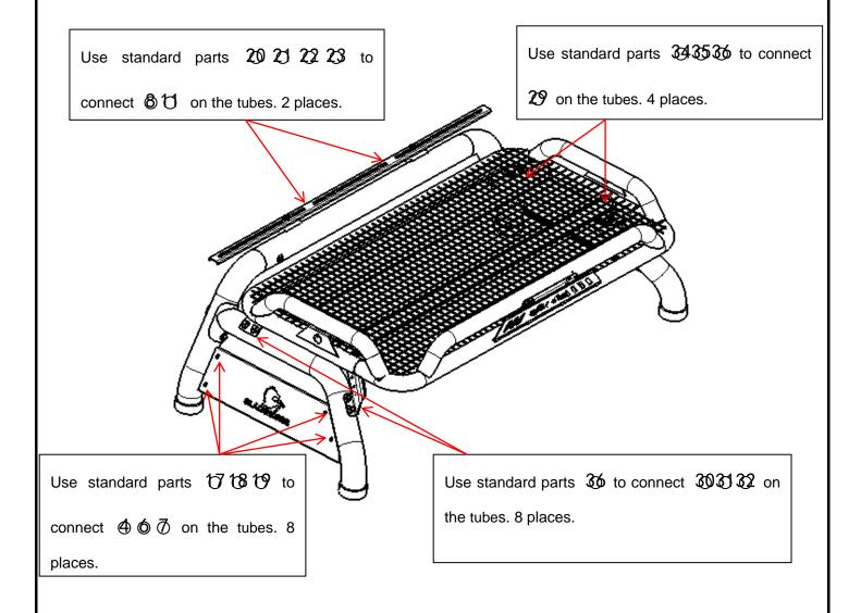
**Step4**: Remove the front and end cover of the support seat. Put the assembled soft tri-fold into the support seat according to the chute, tighten all the standard parts.
