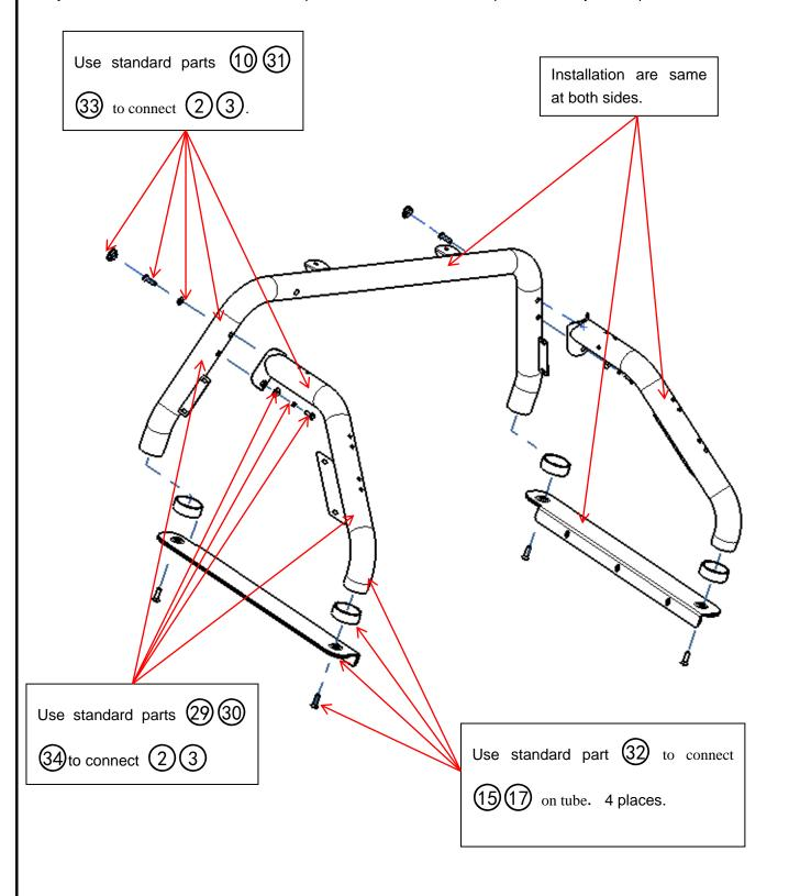
**Step2:** Assemble Luggage frame and tubes with standard parts. Lock all the standard parts after adjust the position.
