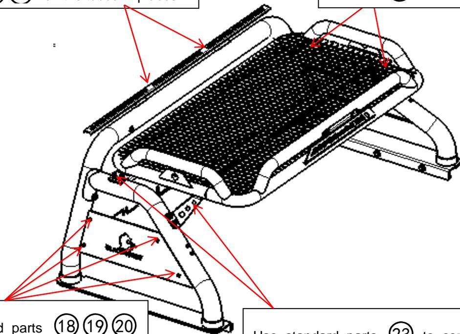
Use standard parts (18) (19) (20) to connect (6) (7) (9) on the tubes. 8 places.
