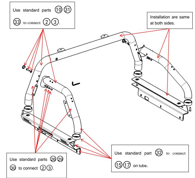
**Step2:** Assemble Luggage frame and tubes with standard parts. Lock all the standard parts after adjust the position.
