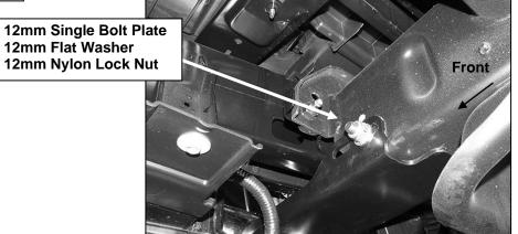
(Fig 11) Passenger Bracket installed in "forward" position to move Bull Bar away from bumper
