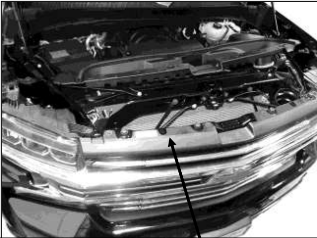
(Fig 5) Remove cover and screws attaching grille
