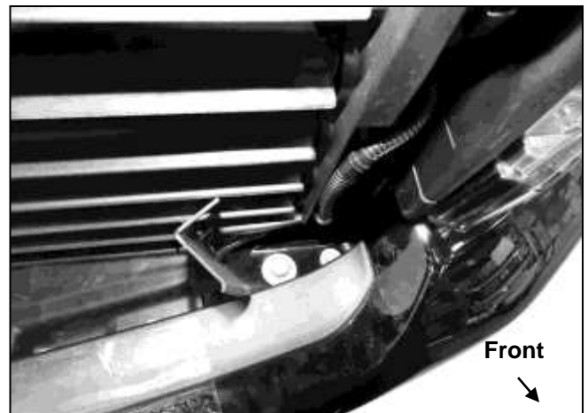
(Fig 8) Pull back cover to locate top bumper bolts
