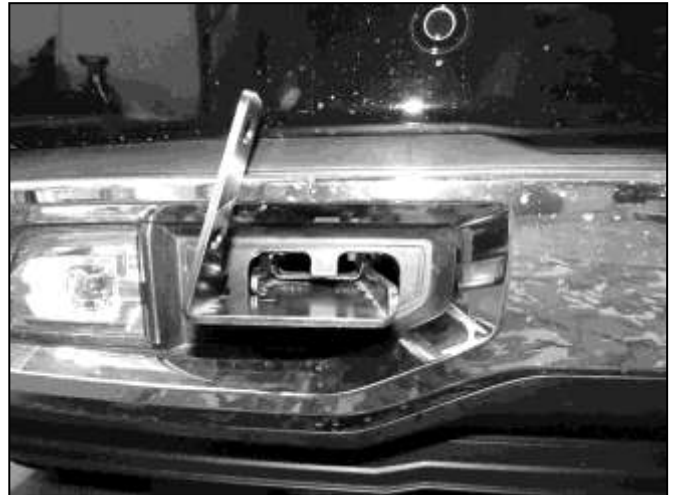
(Fig 18) Passenger/Right side Bracket installed
