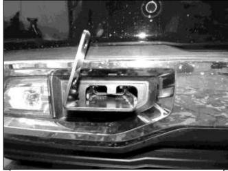
(Fig 18) Passenger/Right side Bracket installed
