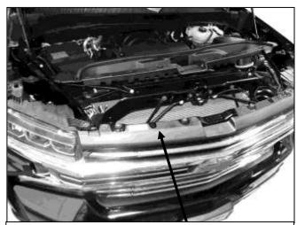
(Fig 5) Remove cover and screws attaching grille
