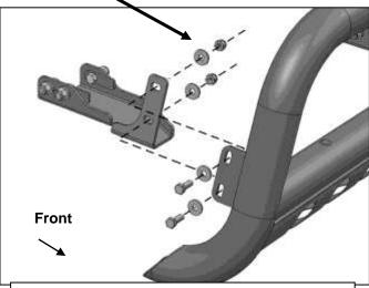
(Fig 19) Attach Bull Bar to outside of Brackets. Passenger/Right side complete installation
