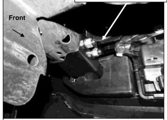
(Fig 15) Outer Passenger/Right side Bracket with Double Bolt Plate pictured from behind bumper
