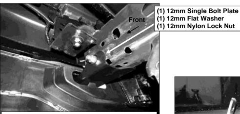
(Fig 17) Inner Passenger/Right side Bracket with Single Bolt Plate pictured from behind bumper
