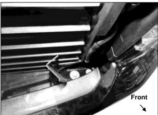
(Fig 8) Pull back cover to locate top bumper bolts
