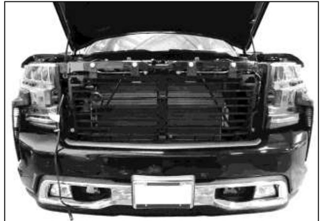
**(Fig 6) Firmly pull grille straight out from vehicle**
