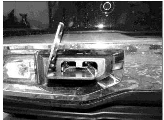
**(Fig 18) Passenger/Right side Bracket installed**
