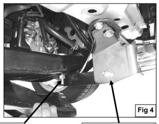
12mm x 90mm Hex Bolt 12mm Nylock Nut 12mm Fender Washer (top) 12mm Flat Washer (bottom)
