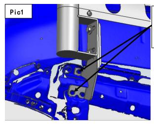
Use the factory hardware to install the bracket on the bottom, but do not tighten up.
