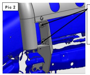
Refer to Pic 2 to install (3), (4) on these holes with (4), (5) and (6), but do not tighten up.
