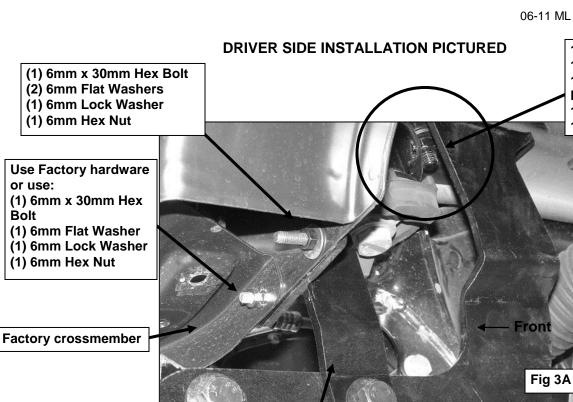
(1) 6mm x 30mm Hex Bolt (1) 6mm Flat Washer (1) 6mm Lock Washer
