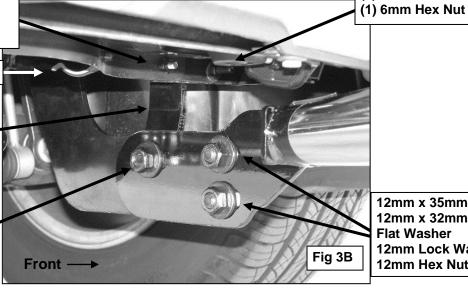
12mm x 35mm Hex Bolt 12mm x 32mm Large **Flat Washer** 12mm Lock Washer 12mm Hex Nut
