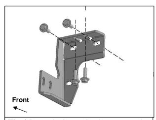
(Fig 2) Reuse the factory hardware to attach the Passenger/Right Mounting Bracket to the frame and inner impact bumper
