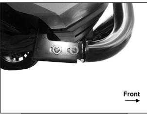
(Fig 10) Attach Bull Bar to the inside of the Mounting Brackets
