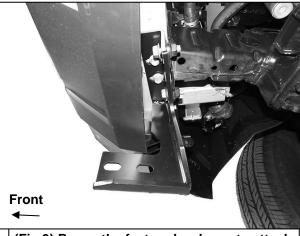
(Fig 3) Reuse the factory hardware to attach the Passenger/Right Mounting Bracket
