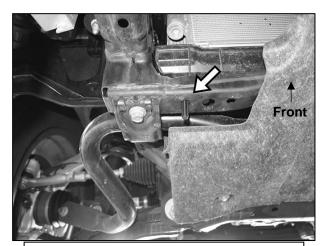
(Fig 6) Pull the Fish Wire with Bolt Plate down and out through the smaller hole in the crossmember then remove Fish Wire
