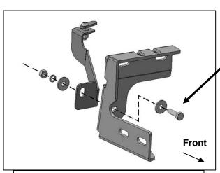
(Fig 8) Attach Support Bracket to back of the Passenger/Right Mounting Bracket
