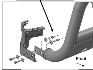
(Fig 9) Attach the Bull Bar to the (2) Mounting Brackets
