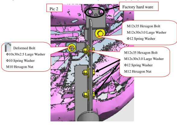
Step 4: Check if all hard ware are installed and then tighten all to complete the installation.
