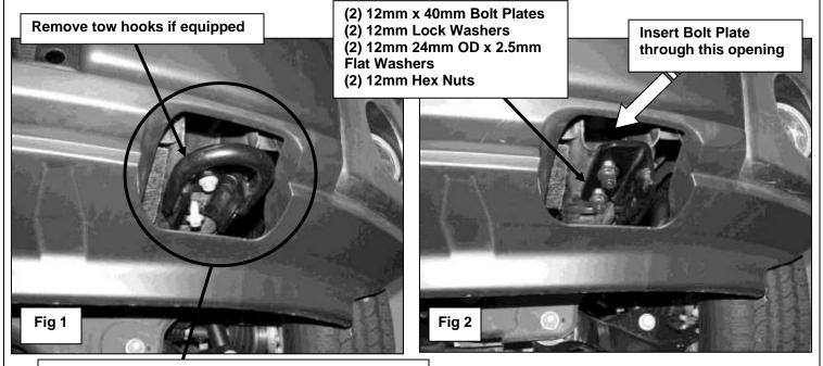
NOTE: On vehicles without tow hooks, the area circled above may be covered by an indented plastic panel. Cut or remove the panel as required to gain access to the front of the frame rail to allow bottom brackets to pass through the bumper cover.
