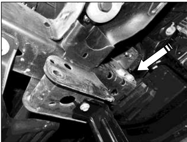
(Fig 3) Passenger/right outer mounting bolts for tow hook pictured from behind bumper
