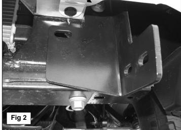
Insert 12mm Spacer Washer between the Mounting Bracket and the frame
