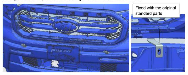
Step 5: Find out the inner radar plastic bracket from the front runner (or from the radar bracket).
