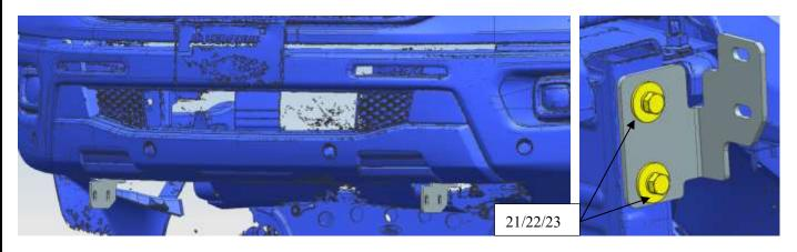
Step 4: Place the brace brackets through the bottom of the plastic grille guard and then fixed with the original standard parts. The left and right side installation are consistent.
