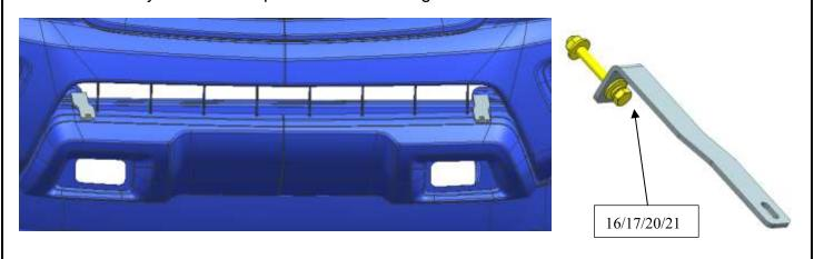
Step 5: Find out the inner radar plastic bracket from the front runner. Then fasten the original radar on the front runner as the ballow shown.
