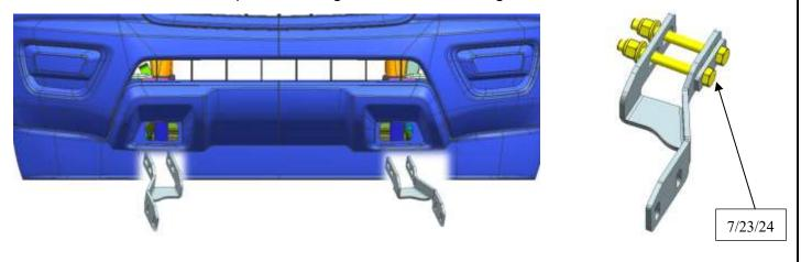
Step 4: Place the brace brackets through the plastic grille guard and then fixed in the rear of the collision beam by the standard parts. The left and right side installation are consistent.
