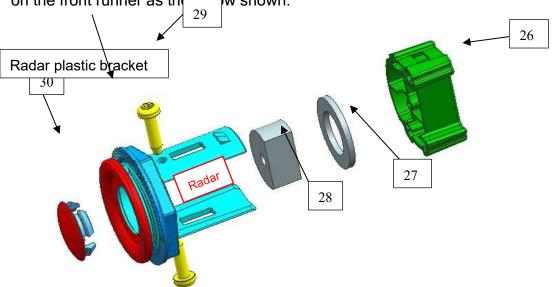
Step 6: Use standard parts to install the front runner with brackets and Brace brackets as the INSTALLING PICTURE shown.
