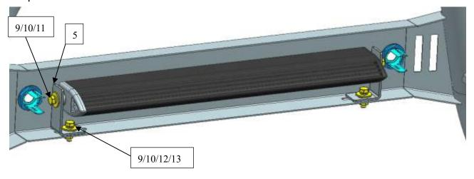
Step 3: Remove the lower factory splash guard before install brackets. Use standard parts and the original standard parts to fasten the left and right brackets on the girder.
