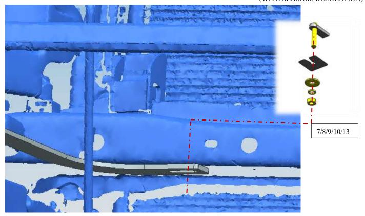
Step 5: Find out the inner radar plastic bracket from the front runner. Then fasten the original radar on the front runner as the below shown.
