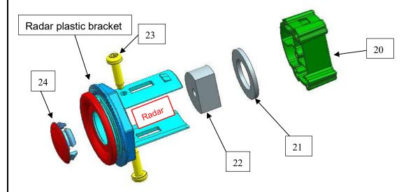
Step 6: Use standard parts to install the front runner with brackets and Brace brackets as the INSTALLING PICTURE shown.
