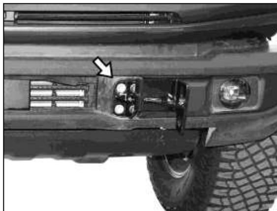
(Fig 4) Models with plastic bumper cover (see Fig 1), reuse the (2) OEM hex bolts to attach the driver/left Mounting Bracket to the front of the bumper (arrow)
