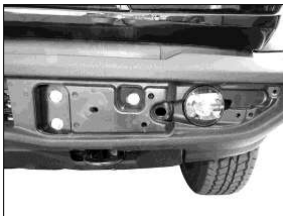
(Fig 2) Models with plastic bumper cover (see Fig 1), remove bumper pads from bumper (driver/left side pictured). Note, unplug parking sensors if equipped
